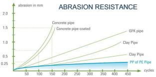
Abrasion curve of various pipe materials according to the Darmstadt procedure
